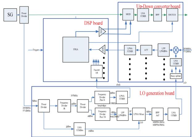
Figure 5: The function block of XFEL LLRF.
