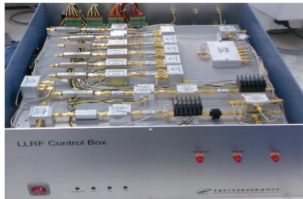
Figure 1: The first generation LLRF controller.
