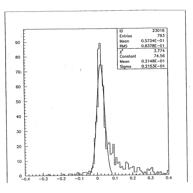
Figure 8: The fractional energy error  $\frac{E(measured)_{jet} - E(reconstructed)_{jet}}{E(measured)_{jet}}$  for a cone of radius R = 0.6 for an iron calorimeter ( $\frac{\epsilon_h}{\epsilon_e} = 1.25$ ). We have used an energy smearing  $= dE = 70\%\sqrt{E} \oplus 2\% \oplus b(e/h)$ . We have corrected the response by multiplying the energy measured in each tower by  $\frac{\epsilon}{\pi}$  (Groom's formula).
