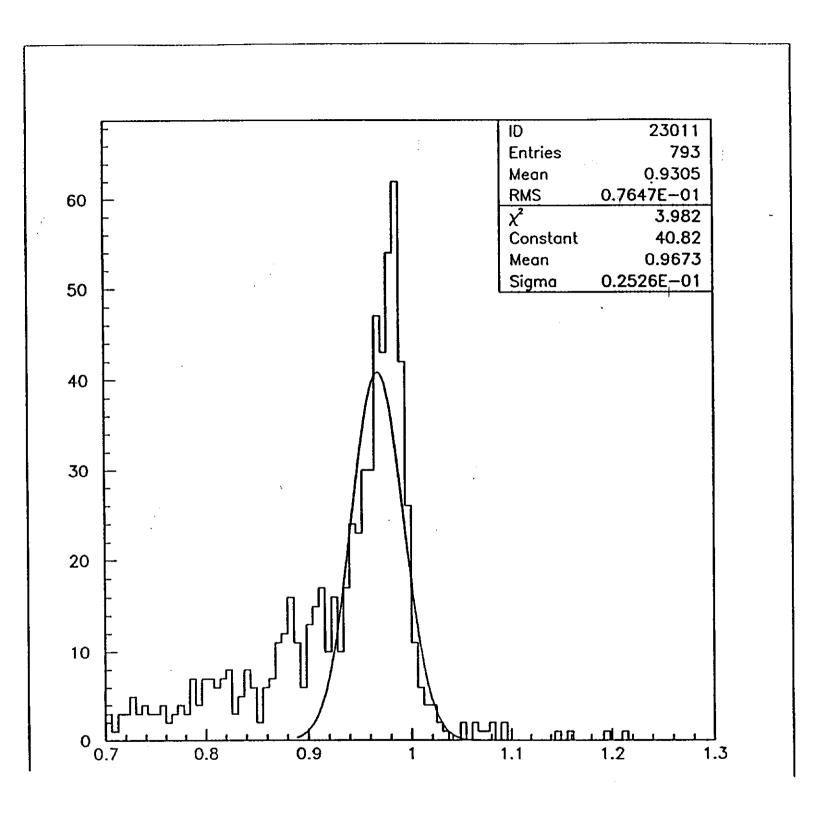
Figure 3: The ratio of the reconstructed mass to the generated mass for a 10 TeV Z'. Our simulation is for a lead hadron calorimeter. We have used an energy smearing  $dE = 70\%\sqrt{E} \oplus 2\%$ .
