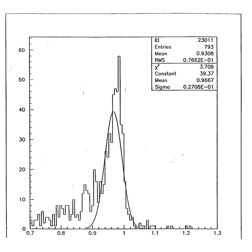
Figure 7: The ratio of the reconstructed mass to the generated mass for a 10 TeV Z'. Our simulation is for an iron calorimeter ( $\frac{\epsilon_h}{\epsilon \epsilon} = 1.25$ ). The energy smearing used was dE =  $70\%\sqrt{E} \oplus b(e/h)$ . We have corrected the response by multiplying the energy measured in each tower by  $\frac{\epsilon}{\pi}$  (Groom's formula).
