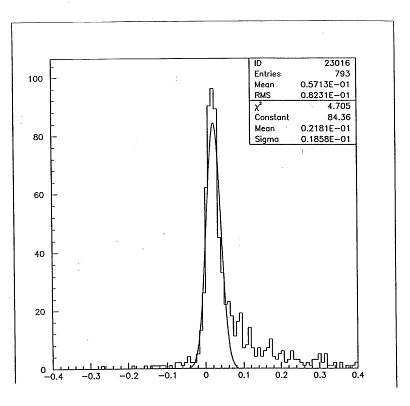
Figure 4: The fractional energy error  $\frac{E(measured)_{jet} - E(reconstucted)_{jet}}{E(measured)_{jet}}$  for a cone of radius R=0.6 for a lead hadron calorimeter. We have used an energy smearing  $dE=70\%\sqrt{E}\oplus 2\%$ .
