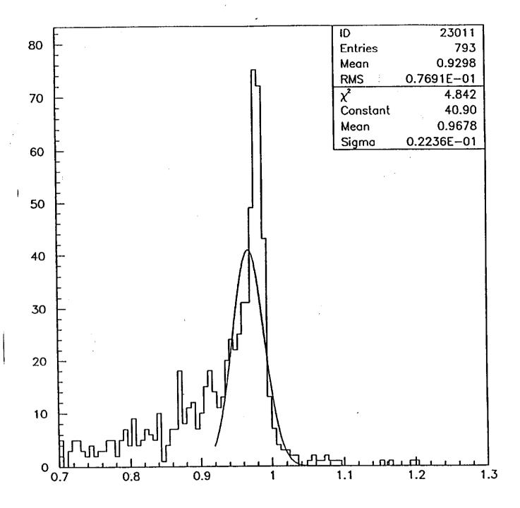
Figure 1: The ratio of the reconstructed mass to the generated mass for a 10 TeV Z'. Our simulation is for an ideal (i.e. no energy resolution) lead hadron calorimeter. The mass is reconstructed in a cone of radius  $R = 0.6 = \sqrt{(\eta)^2 + (\phi)^2}$ .
