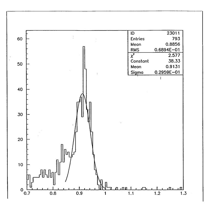
Figure 5: The ratio of the reconstructed mass to the generated mass for a 10 TeV Z'. Our simulation is for an iron calorimeter ( $\frac{\epsilon_h}{\epsilon_e} = 1.25$ ). We have used an energy smearing dE =  $70\%\sqrt{E} \oplus 2\% \oplus b(e/h)$ .
