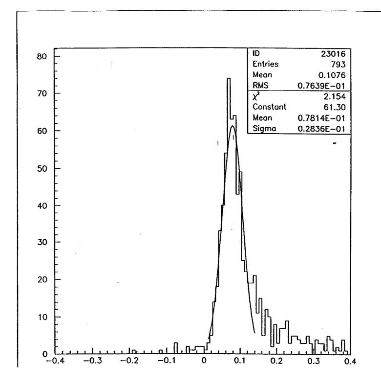
Figure 6: The fractional energy error  $\frac{E(measured)_{jet}-E(reconstucted)_{jet}}{E(measured)_{jet}}$  for a cone of radius R=0.6 for an iron calorimeter ( $\frac{\epsilon_k}{\epsilon_e}=1.25$ ). We have used an energy smearing  $dE=70\%\sqrt{E}$   $\oplus$  2%  $\oplus$  b(e/h).
