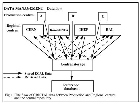
To achieve the physics goals, each part produced, must be of the highest quality and carefully checked prior to its final installation in the detector. As an example, consider the CMS ECAL detector. During the construction phase, physical characteristics will be collected and stored by various laboratories for each part of the detector. This information will need to be centralised in a repository and made available for the calibration of the detector (figure 1.)
