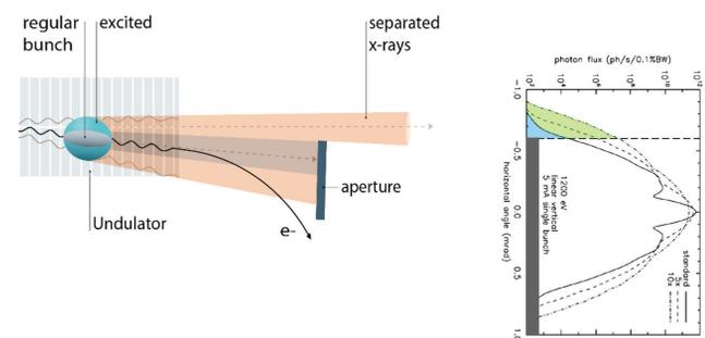
Figure 1: Separation of the MB core from the extended PPRE bunch in the horizontal wings of the undulator cone [3].
