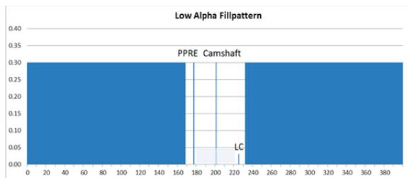
Figure 2: Low- $\alpha$  fill pattern: the short, low current bunch (LC) is positioned at the end of the dark gap to allow pulse separation.
