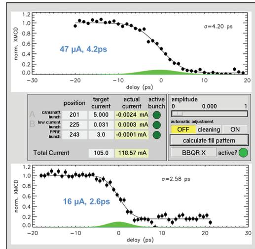
Figure 5: Dialing in bunchlength of 4.2 ps and 2.6 ps by filling the LC bunch with 47  $\mu\text{A}$  and 16  $\mu\text{A}$  resp. The bunch length has been verified with XMCD pump probe measurements, X-ray slicing at the L-edge of a FeGd sample at  $\sigma=65$  fs precision [10].
