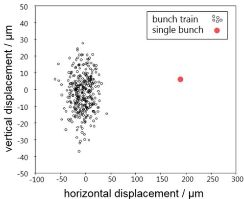
Figure 4: Measured orbit separation of the PPRE excited bunch in low- $\alpha$  mode [9].
