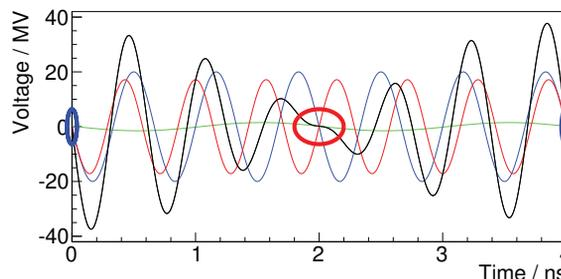
Figure 1: Scheme of the voltage oscillation during one beating period and positions of long (red) and short (blue) bunches, indicated by the colored ellipses. The colored sinusoidal oscillations represent the individual voltages, green 0.5 GHz, blue 1.5 GHz and red 1.75 GHz. The black line shows the resulting sum voltage, which defines both the length and position of each bunch.
