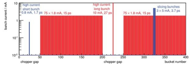
Figure 3: Example of bunch fill pattern with long (red) and short (blue) bunches. There are 400 buckets with 2 ns separation.
