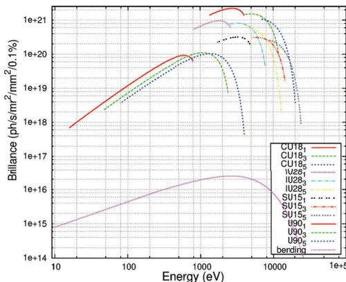
Figure 4: Brilliance spectrum of SR from bending magnets and insertion devices.
