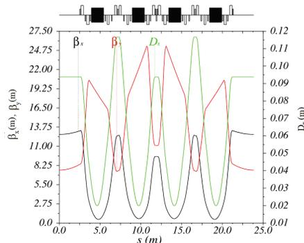
Figure 3: Betatron and dispersion functions in main cell for finite dispersion mode.
