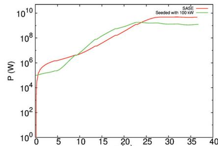
Figure 6: FEL power evaluation along the undulator.
