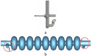
Figure 3: Tesla type HOM coupler (a), 9-cell cavity HOM couplers (b)
