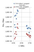
Figure 7:  $Q_{ext}$  (a), transverse shunt impedance  $R_{\perp}$  (b), long shunt impedance  $R_{\parallel}$  (c), for HOM's in 9-cell cavity with cylindrical beam pipes and 9-cell cavity with corrugated beam pipe.
