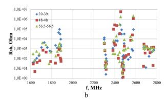
Figure 6: Q<sub>ext</sub> (a), shunt impedance R<sub>sh</sub> (b) for HOM's in 3 types of 9-cell cavity with corrugated beam pipe and different external radius dr1 (39, 48 and 56.5 mm)Results of EDC of three types of cavities with different radius dr1 comparison are summarized in Table 1.
