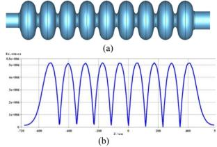
Figure 1: (a) Model of 9-cell cavity with cylindrical beam pipes and (b) electric field distribution for operational mode.
