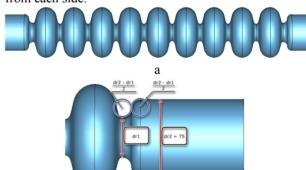
Figure 5: Nine-cell cavity with corrugated beam pipe (a), corrugated beam pipe geometry (b)
