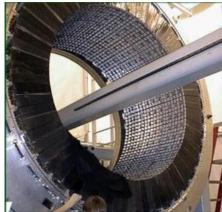
Figure 3.21: Photograph of the barrel portion of the EMC.
