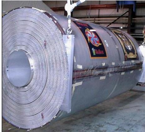
Figure 3.10: Photograph of the DCH. The 40 layers, grouped into 10 *superlayers*, are visible on the forward end of the chamber.
