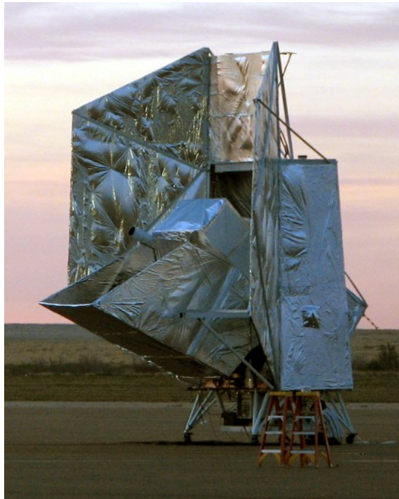
Figure 4.4: The EBEX payload with baffles deployed in Ft. Sumner. In this photo the instrument is standing on the launchpad in an open area to test sidelobe response using an RF source on a crane (not pictured). The large wings and box-like structure on the right make up the outer frame baffling, which prevent sunlight from directly impinging on the inner frame and electronics crates. The central tilted box and open scoop are the inner frame baffles, which move in elevation with the instrument, and reject stray light from the optical path.
