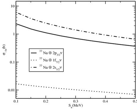
FIG. 1: The total cross-section vs one neutron separation energy for  $^{34}\text{Na}$  breaking on  $^{208}\text{Pb}$  at 100 MeV/u beam energy to form a  $^{33}\text{Na}$  core and a neutron. The deformation parameter,  $\beta_2$  has been set to 0.
