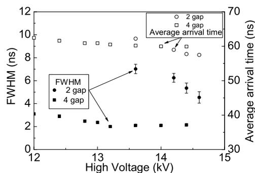
FIG. 2: The time resolution (FWHM) and the average signal arrival time as a function of the high voltage for the two MRPC (one double gap and one 4-gap).
