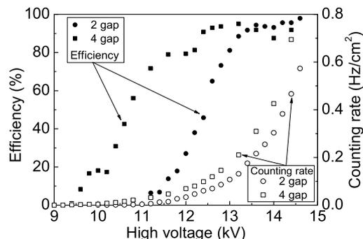
FIG. 1: The efficiency and the counting rate as a function of the high voltage for the two MRPC (one double gap and one 4-gap).
