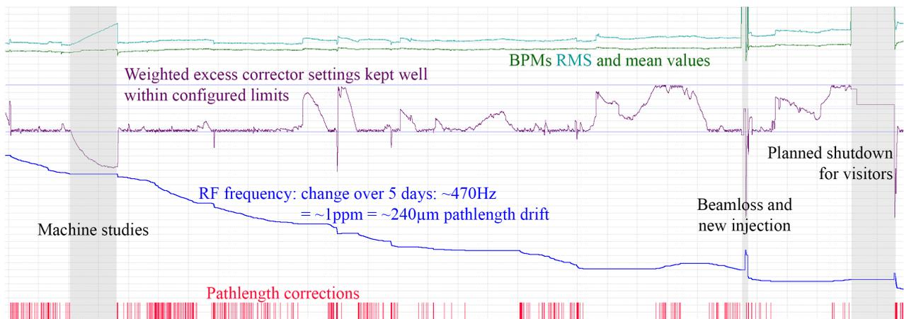
Figure 6: Plot of ~400 path length corrections over 5 days after one week of low current low- $\alpha$  operation. Shown are sum of the weighted excess corrector settings and the resulting RF frequency. BPM RMS and mean values are stable within  $\sim 1 \mu\text{m}$ .
