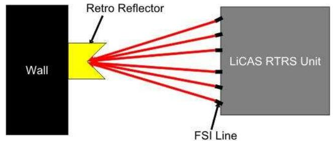
Figure 4: Sketch of External FSI System
