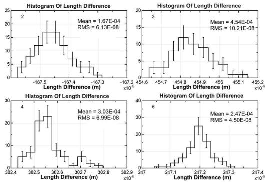
Figure 17: Histogram of the lengths measured by the internal FSI on car 3 with the lengths of line 1 subtracted during a 30 hour period
