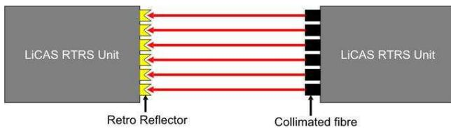
Figure 7: Sketch of the Internal FSI System
