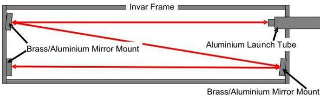
Figure 2: Sketch of a LiCAS Reference Interferometer
