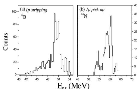
Figure 3. Kinetic energy spectra of (a)  $^{12}\text{B}$  formed in  $1p$  stripping and (b)  $^{14}\text{N}$  formed in  $1p$  pickup in  $^{13}\text{C}+^{93}\text{Nb}$  reaction at  $65\text{MeV}$  energy
