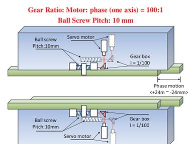
Figure 3: Phase driver mechanism of EPU48.
