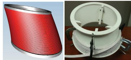
Figure 3: Conceptual drawing (left) and 3d printer version (right) of the Nb<sub>3</sub>Sn HS spool and conductor that will be fabricated and tested in the Fermilab Vertical Magnet Test Facility. The test will use two layers of cable.
