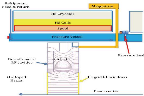
Figure 4: Conceptual diagram showing the features of a beam-cooling module with dielectric-loaded RF cavities, Be RF windows, pressure vessel, HS coil, and its cryostat.
