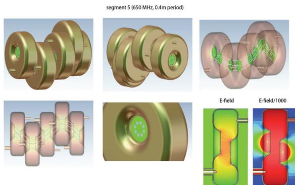
Figure 2. 3D conceptual design and initial simulations for the re-entrant cavities that could be used in mid-section of an HCC.
