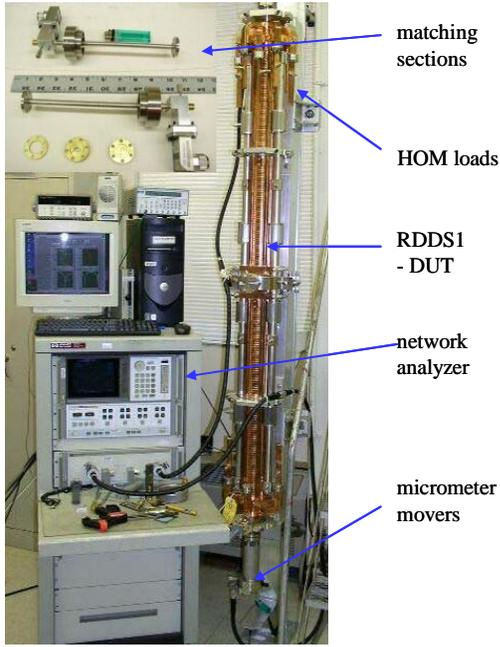
Figure 2: Wire measurement setup.
