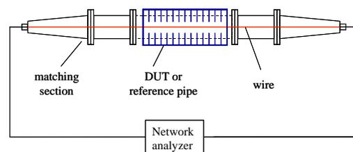
Figure 1: Sketch of the wire measurement setup.
