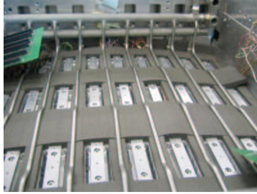
Figure 2.14: Picture of the grid. The connectors are visible, each of them hold 10 channels.
