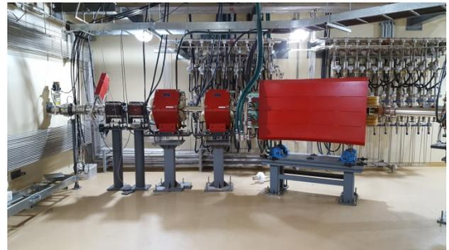
Figure 5: Installed proton beam transport system from 45 degree bending magnet (right) to penetration hole to the target room (left).
