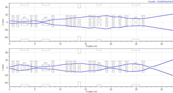
Figure 2: Beam envelope along the beam line.
