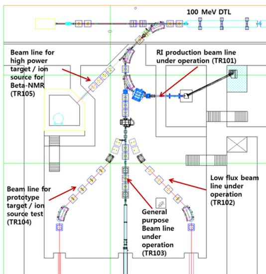
Figure 1: Layout of KOMAC 100-MeV proton beam line.
