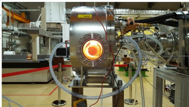
Figure 6: Prototype target ion source off-line heating test.
