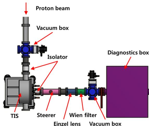
Figure 7: Schematics of the <sup>8</sup>Li beam transport system.
