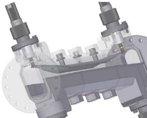
Figure 7: DAΦNE new injection kickers (Courtesy D.Alesini)
