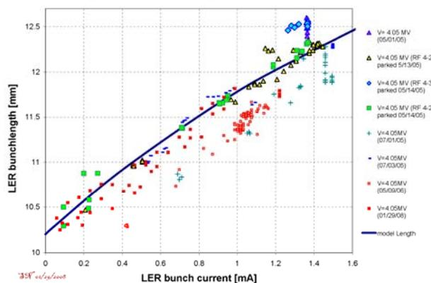
Figure 2: LER bunch length as a function of a bunch
