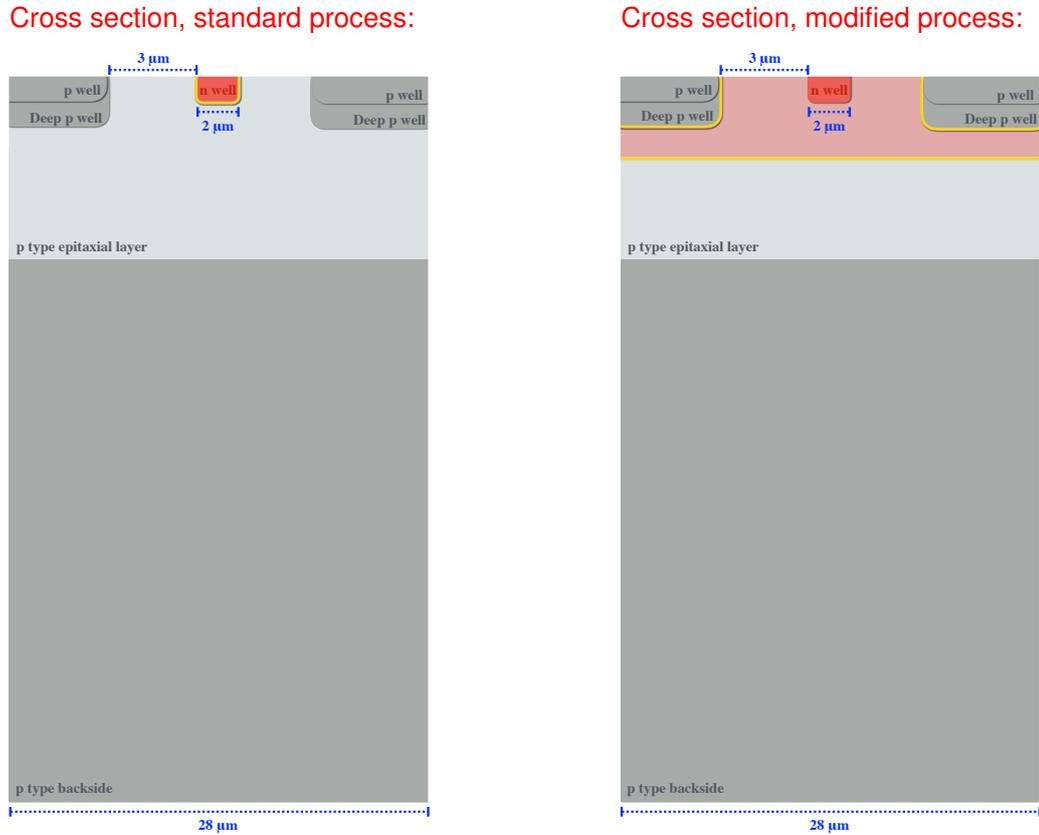
Figure 7.4: Schematic of the simulated cross section of a single pixel cell for the *standard process* (left) and the *modified process* (right), with the pn junctions marked in yellow (not to scale). The colour intensities illustrate the doping levels: lower doping levels are indicated by a lighter colour.
