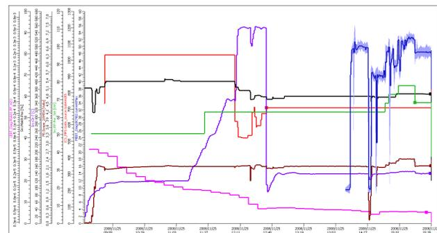
Figure 4: H<sub>2</sub>O partial pressure (pink), Cs Collar temperature (purple), 2 MHz power (green), matching capacitance (black), antenna current (brown), pulse length (red), and maximum beam current (blue) during the conditioning, cesiation, and tune up of a source.
