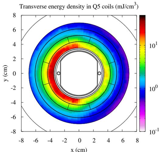
Figure 3: Simulated transverse energy density distribution in the Q5.R6 coils at the position where the maximum energy deposition of  $\sim 33 \text{ mJ/cm}^3$  occurs.
