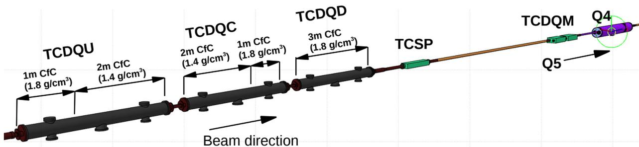
Figure 1: FLUKA model of the IR6 insertion region, from the TCDQ to the MQY.4R6 (Q4). The Cfc-absorber blocks of the TCDQ with a lower density of  $1.4 \text{ g/cm}^3$  are located around the shower maximum in the absorber.
