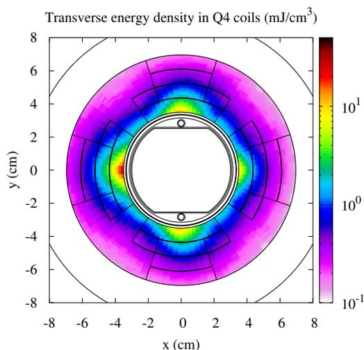
Figure 2: Simulated transverse energy density distribution in the Q4.R6 coils at the position where the maximum energy deposition of  $\sim 22 \text{ mJ/cm}^3$  occurs.
