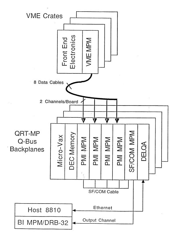
Fig. 1: DØ Data Acquisition Hardware Layout
