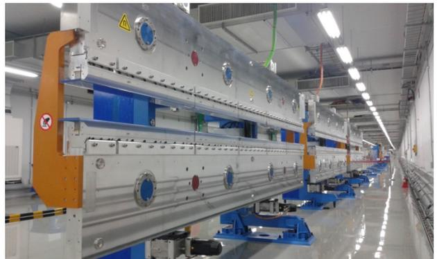
Figure 9: Installed undulator in undulator hall.
