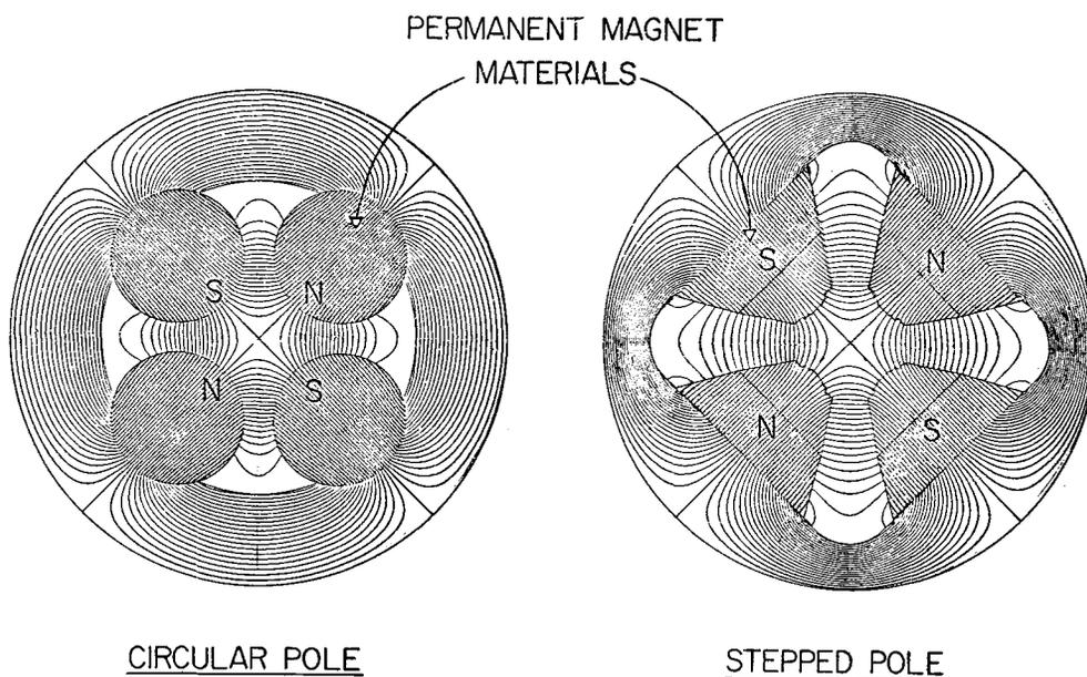
Fig. 5. Permanent magnet quadrupole lens geometries and calculated fields.
