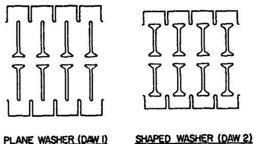
Fig. 3. Disk and washer structure (two models).
