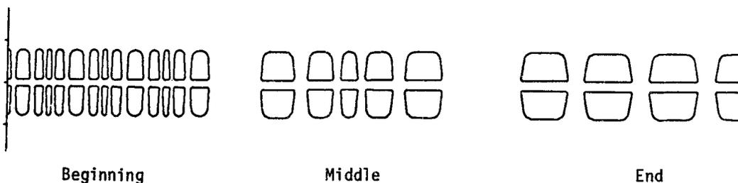
Fig. 1. Selection of drift tube profiles for the PIGMI Prototype.
