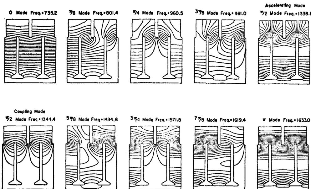
Fig. 4. Family of modes from the disk and washer mode spectrum.
