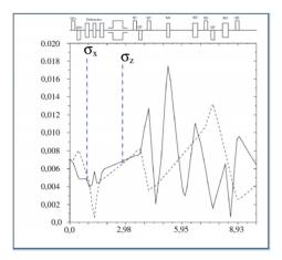
Figure 6: MAD simulation of the transverse beam dynamics of the transfer line. Shown are the horizontal and vertical beam width  $\sigma_x$  and  $\sigma_z$  versus the position in the transfer line.
