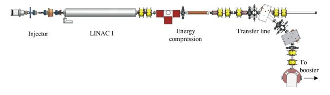
Figure 1: Overview of the new injection system which will be installed at the linear accelerator LINAC I at ELSA.
