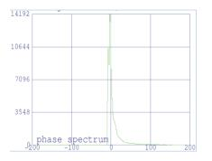
Figure 4: Bunch length after the travelling wave buncher. Shown is the number of particles versus the phase position of the particles relative to the main particle.
