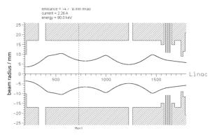
Figure 5: Simulation of a 2 A beam propagating through the beam guiding elements based on the paraxial equations.
