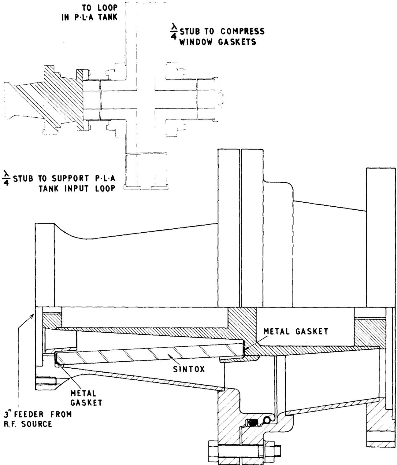
COAXIAL SINTOX WINDOW FOR R.F. INPUT
