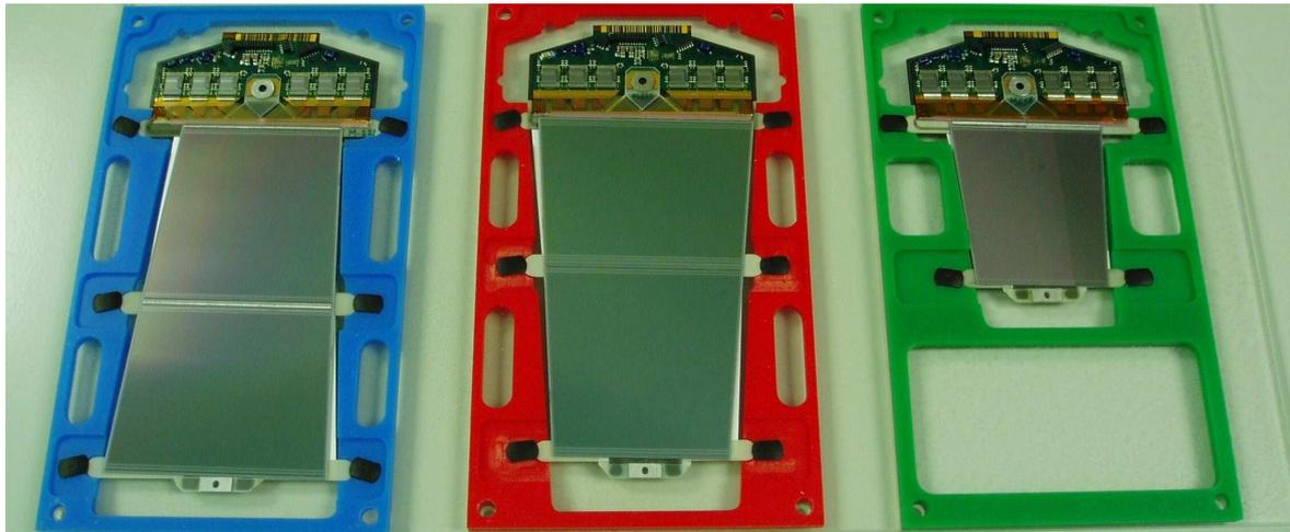
**Figure 4.2:** Three types of modules assembled on the ATLAS SCT endcaps, showing the layout of the five different wedge-geometries of the endcap sensors (taken from Ref. [64]). Each module consists of two back-to-back sensor layers, rotated with respect to each other by  $40\text{ mrad}$ . From left to right: Outer module, Middle module and Inner module. The readout electronics are mounted on hybrids at the ends of the modules.
