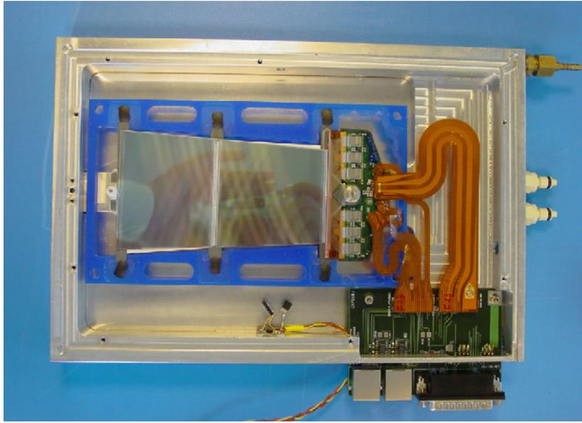
**Figure 4.12:** Photograph of an Outer endcap module supported by its transport frame inside its aluminium test box (taken from Ref. [77]). The dry air and coolant inlets are visible, as well as the patch card and the kapton cables.
