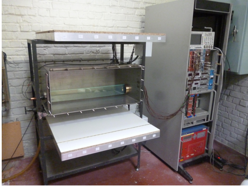
FIGURE 3.1: Picture of the Cherenkov detector (on the left) together with the readout electronics (on the right). The water tank is empty and opened to show the positioning of the wavelength shifter inside. Two bins containing the trigger scintillation counters are placed above and below the watertank.
