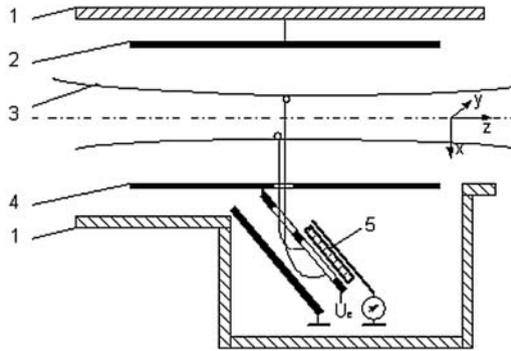
**Fig. 15.9.** Beam profile monitor using residual-gas ionization: 1, beam line wall; 2, grounded condenser plate; 3, ion beam; 4, extraction condenser plate connected to deflecting plate of electrostatic mirror; 5, channel-plate amplifier of electron–optical converter
