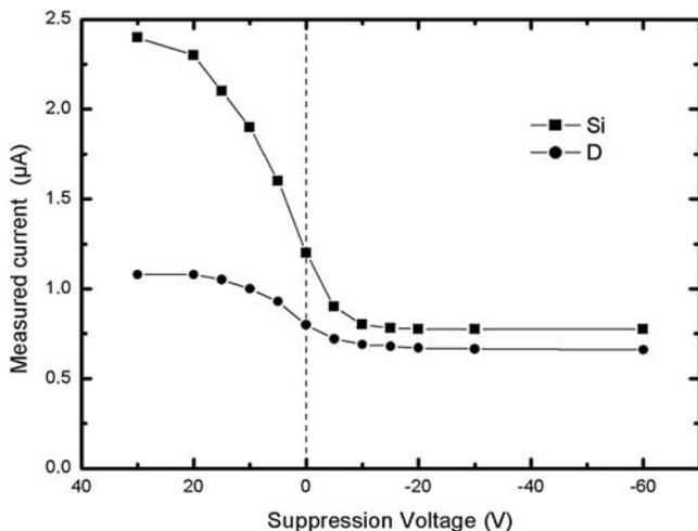
**Fig. 15.3.** Dependence of the measured beam current on the suppression potential for 0.7 MeV  ${}^2\text{H}^+$  and 3 MeV  $\text{Si}^{2+}$  ions. The beam currents at positive suppression voltages indicate the different secondary-emission efficiencies
