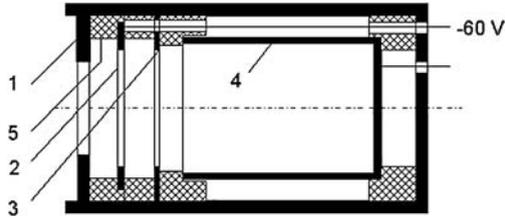
**Fig. 15.1.** Faraday cup with electrostatic suppression: 1, entrance aperture; 2, suppression electrode; 3, grounded separation electrode; 4, measuring cup
