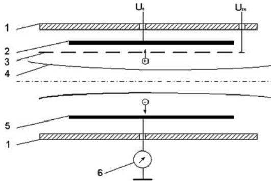
**Fig. 15.4.** Principle of beam current measurement using residual-gas ionization: 1, beam line wall; 2, extraction electrode; 3, secondary suppression electrode (optional); 4, ion beam; 5, collecting electrode; 6, current measurement
