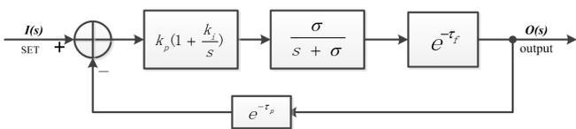
Fig. 4. The feedback model of the transfer function.
