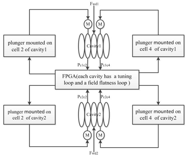
Fig. 5. Diagram of the tuning loops and field flatness loops at SSRF booster.
