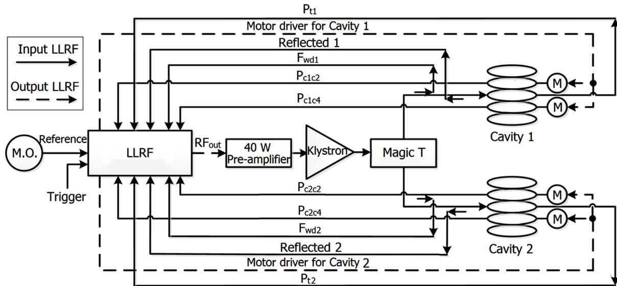
Fig. 1. Layout of the RF system of SSRF booster. The RF signals sampled and processed by the LLRF controller include the reference signal, forward power signal  $F_{wdi}$ , reflected power signal Reflected  $i$ , pick-up signals from  $P_{cic2}$ ,  $P_{ti}$  and  $P_{cic4}$  ( $i$  denotes cavity number of the 5-cell copper cavities). M.O., master oscillator; Trigger, the timing with a repetition rate of 2 Hz.
