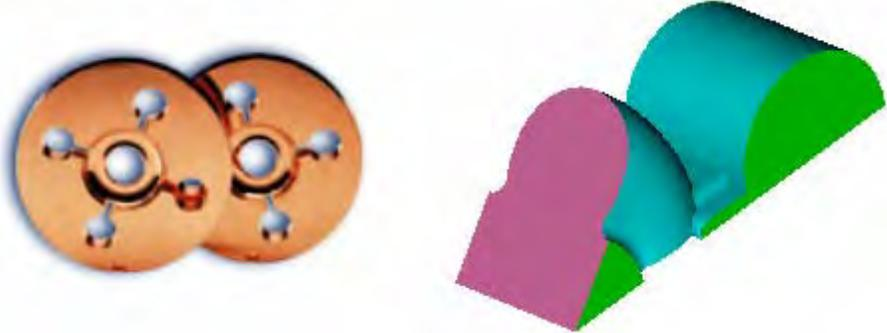
**Figure 1.** Single cell of the Round Damped Detuned Structure RDDS-1 cavity proposed for the NLC (1/8 model). Photograph courtesy of K. Ko, SLAC.
