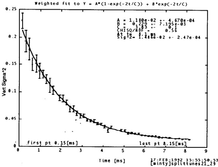
Figure 1. NDR Synchrotron light camera: beam size vs. time
