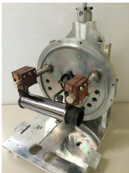
Figure 1. The SPES Target-Ion Source Unit, without the water cooled aluminum cover.
