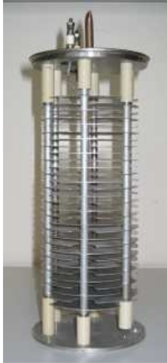
Figure 2.6: BLM ionization chamber developed for SPS. Metallic enclosure removed.
