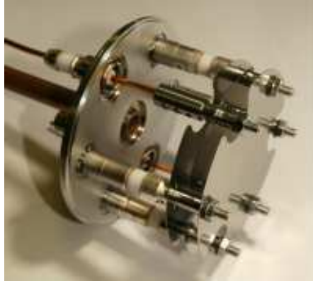
Figure 2.7: Secondary emission monitor. Metallic enclosure removed.
