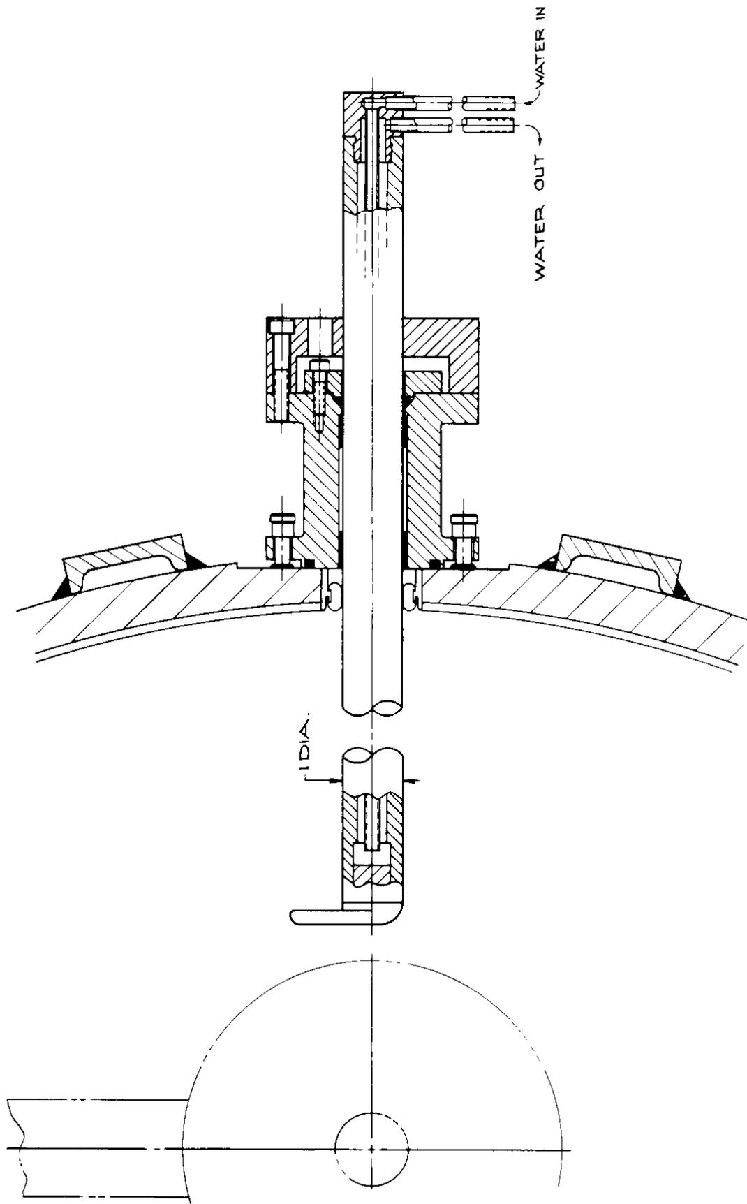
Fig. 6. Post coupler in operating condition.
