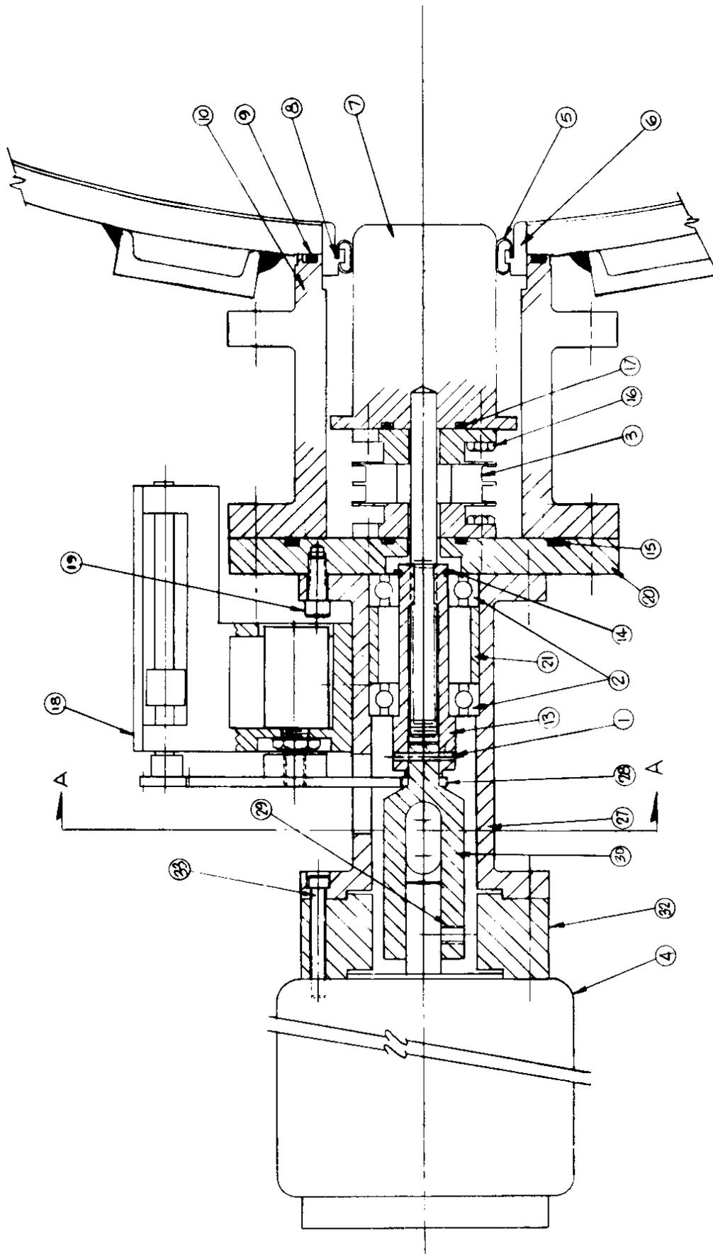
Fig. 9. Motorized tuner - cavity 1.
