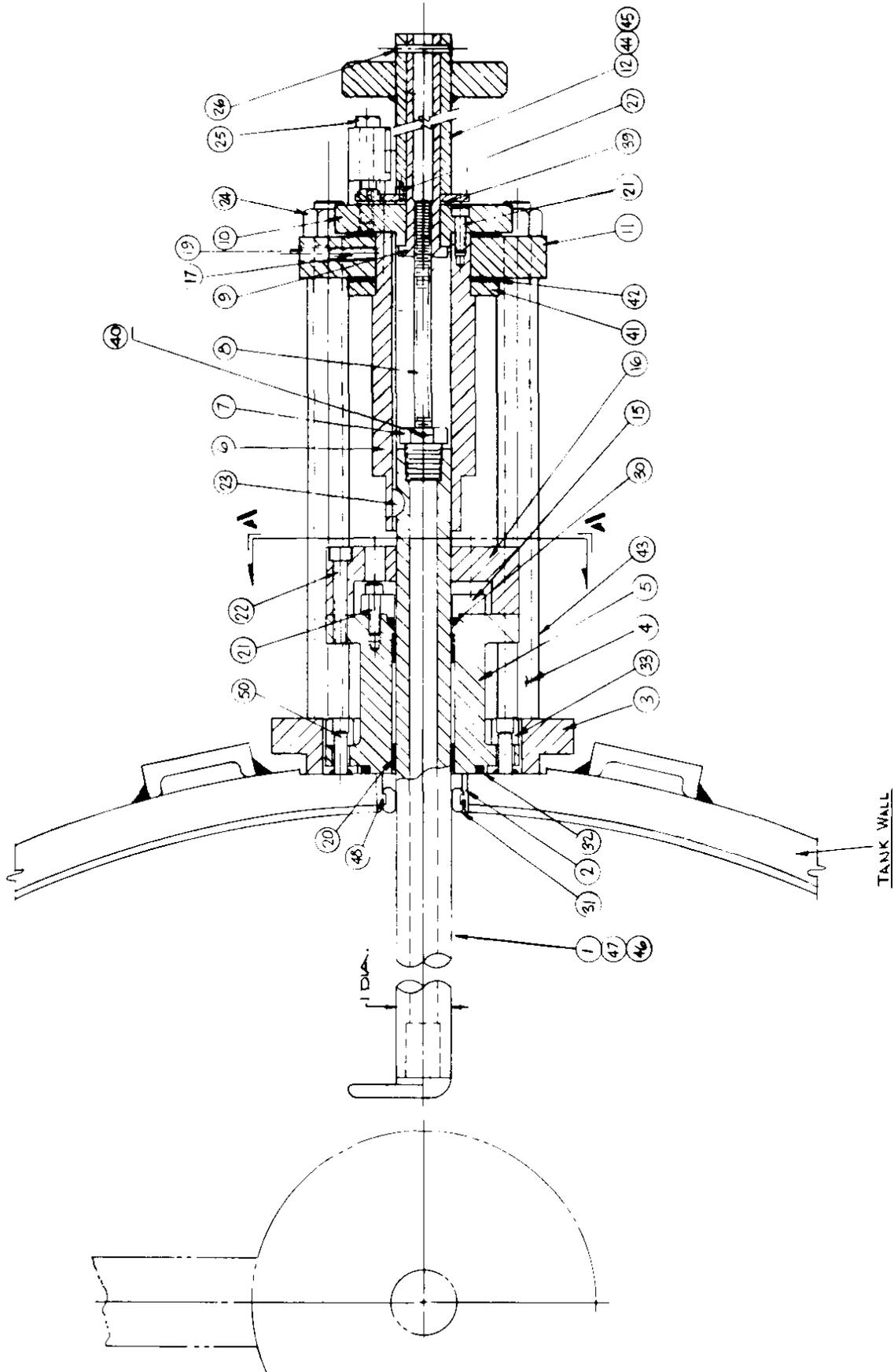
Fig. 5. Post coupler with adjusting mechanism.
