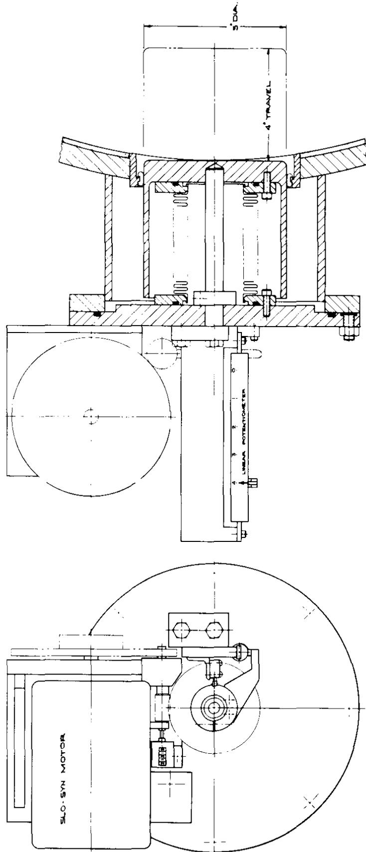
Fig. 8. Motorized tuner--cavity 2 through 9.
