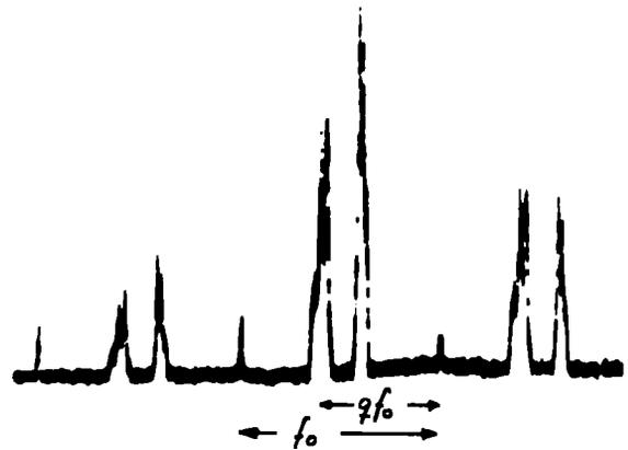
Fig. 1 - Frequency spectrum of the difference signal derived from two plates and induced by the Schottky noise in the beam. Small peaks harmonics of the revolution frequency. Large peaks fast and slow transverse waves.
