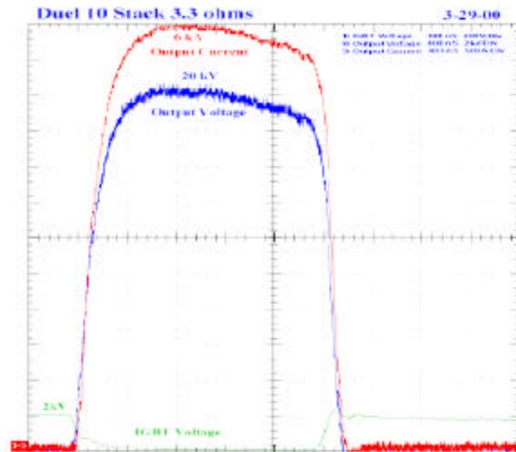
**Figure 4.** Ten-Stack Test Results into 3.3 Ohm Load.
