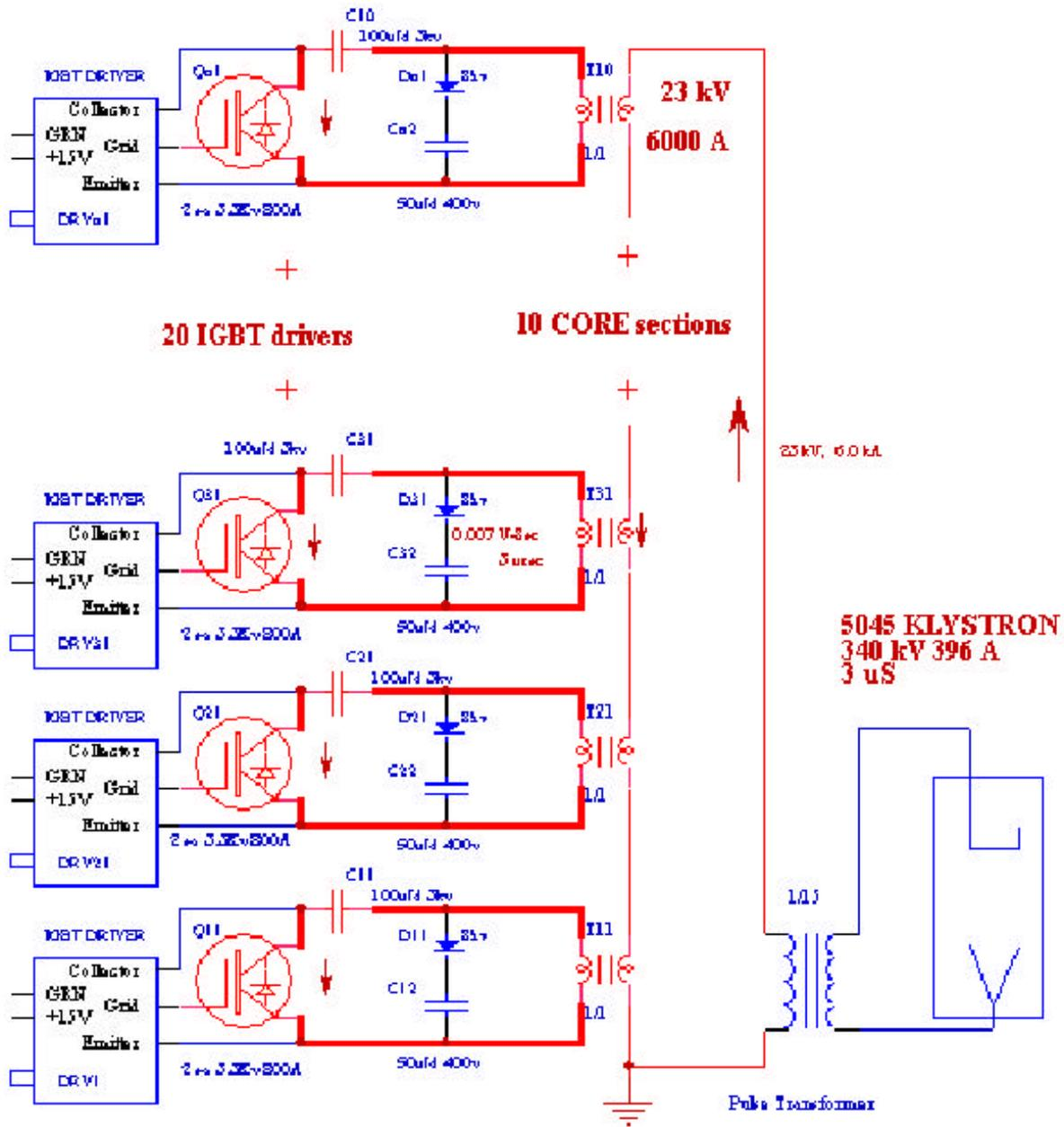
Figure 6. Ten stack modulator schematic.
