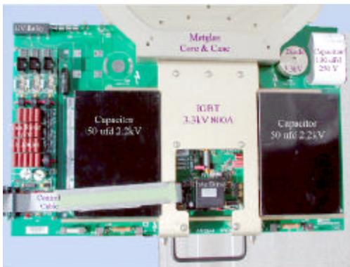
Figure 2. Driver board with partial view of core case.
