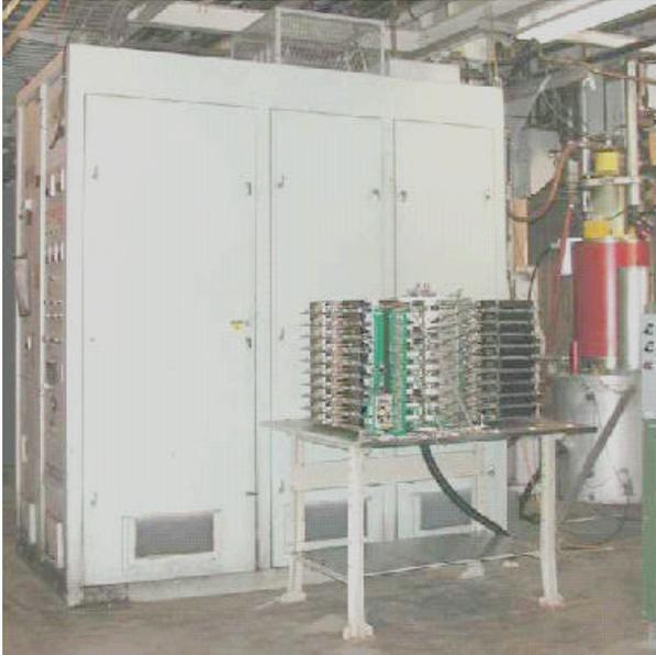
**Figure 3.** Ten-Stack Modulator (in foreground) with the PFN Modulator and 5045 Klystron.
