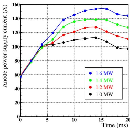
Figure 4: Calculated current of the anode power supply on several beam power during acceleration. Black line: 1.0 MW-eq. beam; red line 1.2 MW-eq. beam; green line: 1.4 MW beam; blue line: 1.6 MW-eq. beam. The cavity uses FT3L ( $10\mu\text{m}$ ) cores at resonance frequency of 2.5 MHz.
