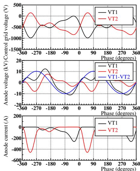
Figure 3: Tube operation analysis result of 1.6 MW-eq. beam acceleration in which the cavity uses FT3L (10 $\mu\text{m}$ ) cores at the resonance frequency of 2.5 MHz.
