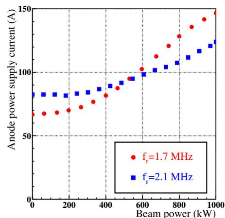
Figure 1: Measured beam power dependence of the anode power supply current. Red circle: cavity resonance frequency of 1.7 MHz; blue square: cavity resonance frequency of 2.1 MHz.
