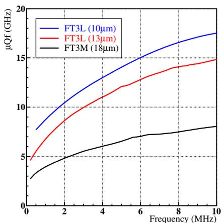
Figure 2: Measured frequency dependence of  $\mu\text{Qf}$  product. Black line: FT3M with 18  $\mu\text{m}$  ribbon; red line: FT3L with 13  $\mu\text{m}$  ribbon; blue line: FT3L with 10  $\mu\text{m}$  ribbon.
