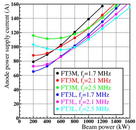
Figure 5: Calculated beam power dependence of the required anode power supply current on several cavity conditions.
