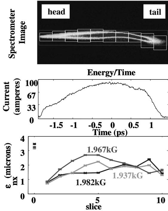
Figure 2: Slice emittance data from the GTF for three gun solenoid fields.
