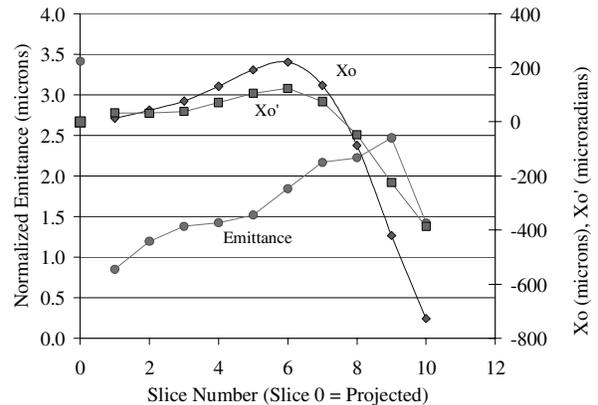
Figure 5: The slice offset in position and angle in front of the quadrupole doublet at 300 pC and a solenoid field of 1.982 kG. Slice 0 is the projected emittance and by definition the offset of the projected beam is 0.
