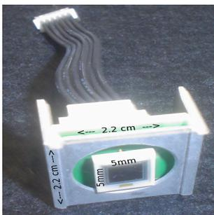
(e) APD + CSP glued together and the flatband cable for connection to the T-card
