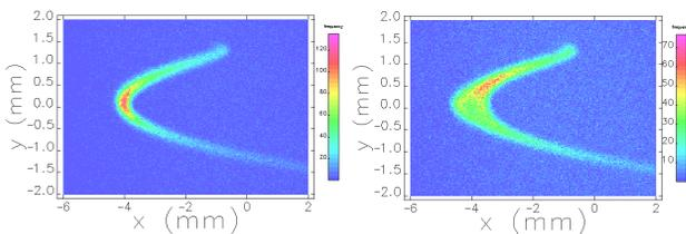
Figure 4: Beam image after the energy spectrometer with laser off (left) and on (right), from simulation. The peak energy modulation is 30 keV.
