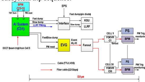
Figure 2: Post Mortem configuration diagram.
