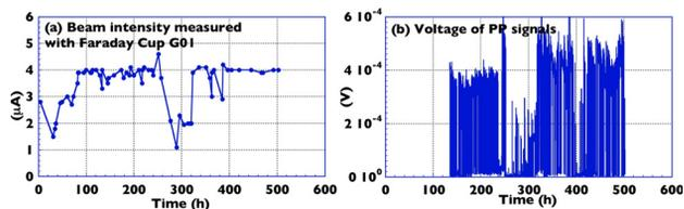
Figure 2: Stability of 345 MeV/nucleon  $^{48}\text{Ca}$  beam extracted from SRC. Observed beam intensity measured with a Faraday cup is shown in (a). Points show measured values; the line is only a guide for the eye. Beam bunch signals measured with a phase-pick (PP) electrode are continuously analysed with a lock-in amplifier. Voltages of the second harmonic component of the signals are shown in (b). A decrease in beam intensity around  $T = 300$  h was caused by a user's request.
