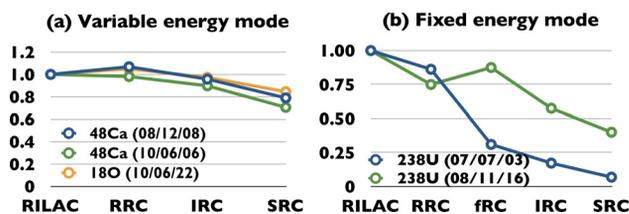
Figure 1: Transmission efficiency of RIBF cyclotron complex. Output intensity of the cyclotrons relative to that of injector RILAC is shown. Charge-stripping efficiency is excluded from the present plot. Error from beam intensity monitors is thought to be 10% and is not calibrated in the present plot.
