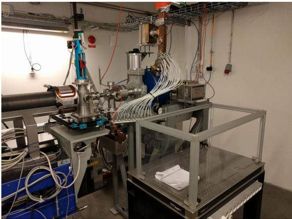
Figure 3: View of the gun, solenoid, start of emittance meter and empty laser table.
