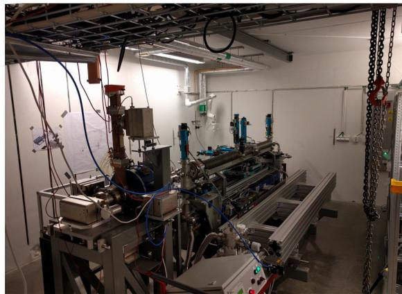
Figure 2: View of the GTF with the gun to the left and emittance meter to the inner left. The second free diagnostic line is on the inner right.
