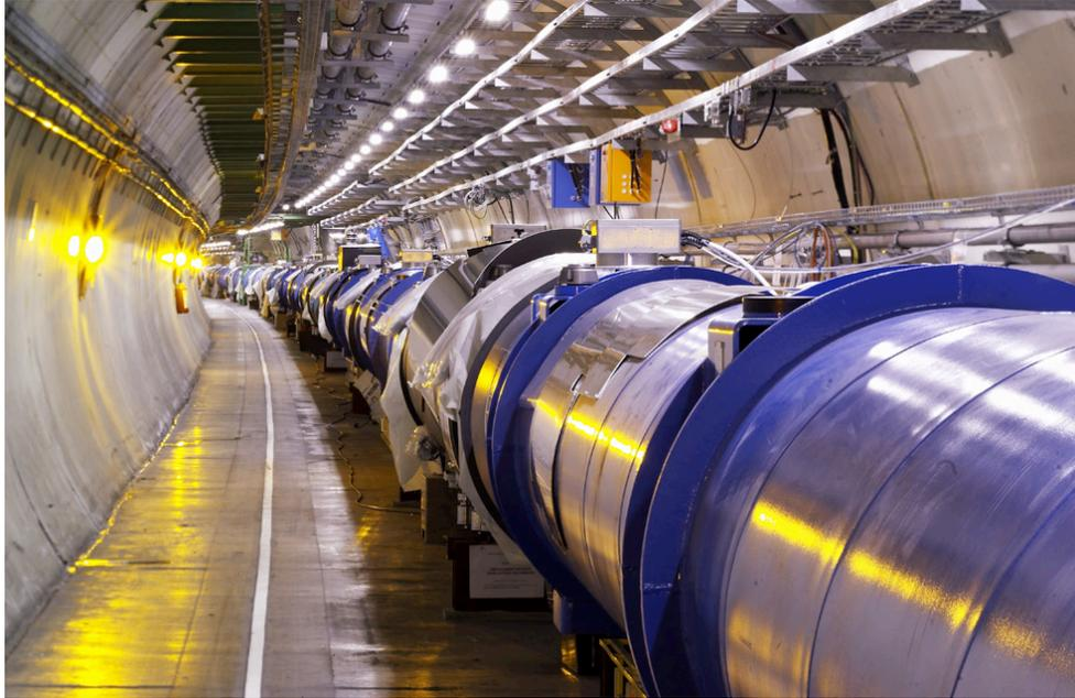
Figure 14: The LHC dipole magnets.
