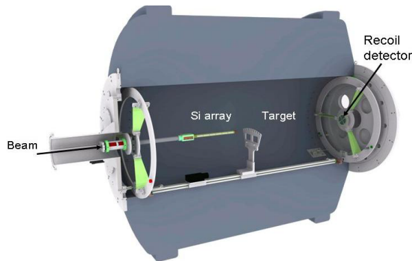
Fig. 5. Computer aided design rendering of the HELIOS spectrometer identifying the beam entrance, the Si detector array that is mounted onto an alignment ring, the target “fan” as well as of the recoil Si detector telescope.
