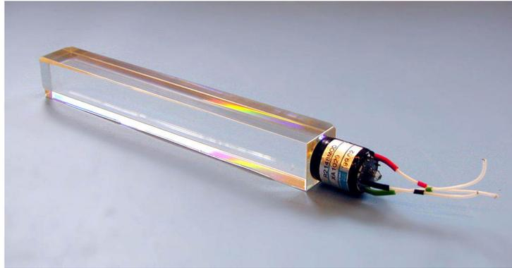
Figure 2.10:  $\text{PbWO}_4$  crystal used in the ECAL with the photo-diode glued to the back of the crystal.
