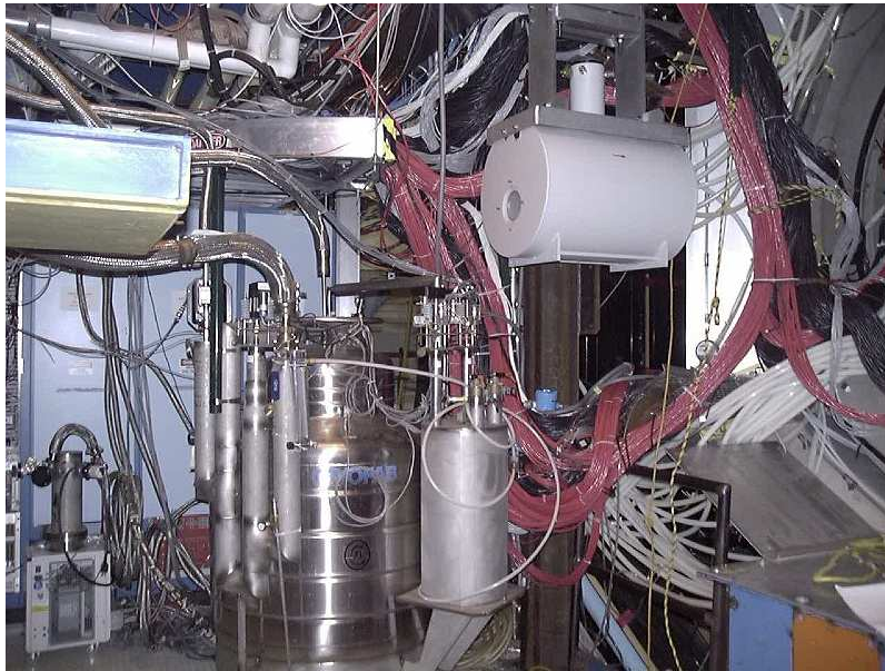
Figure 2.16: The FROST 5 T polarizing magnet is shown here. Figure taken from [71].
