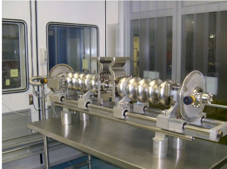
Figure 2.2: A cryomodule cavity shown before installation. Figure taken from [71].
