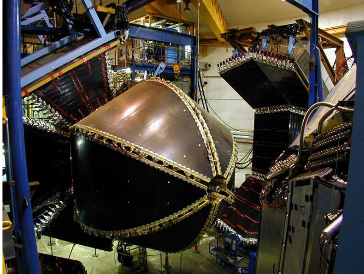
Figure 2.4: The inside of Hall B with CLAS spread open for servicing. The round item in the middle is the outer face of the Region 3 drift chamber. The TOF detectors surround the chambers during physics running. Figure taken from [71].
