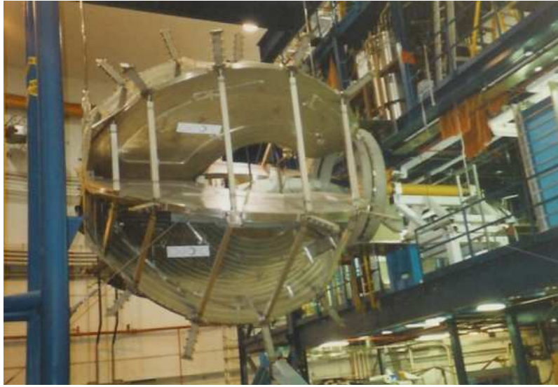
Figure 2.9: The CLAS torus coils in Hall B prior to detector installation. Figure taken from [71].
