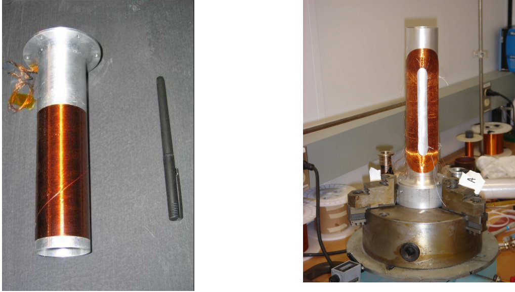
Figure 2.20: The holding coils used in the FROST experiment. (a) The holding coil for the longitudinally polarized target and (b) the holding coil for the transversely polarized target. Figures taken from [87].
