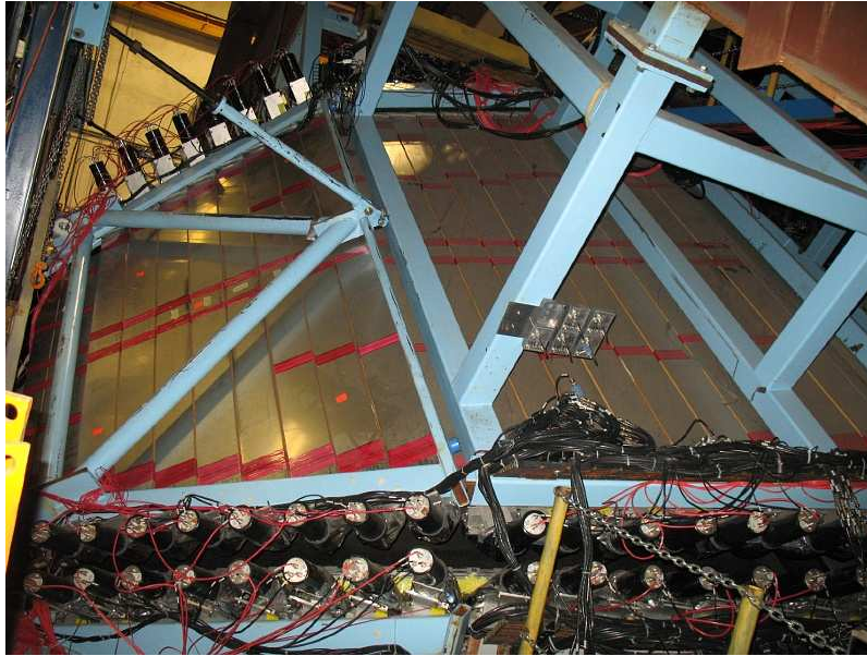
Figure 2.13: The outer portion of the TOF system paddles are shown here with PMTs attached to either end of the paddle.
