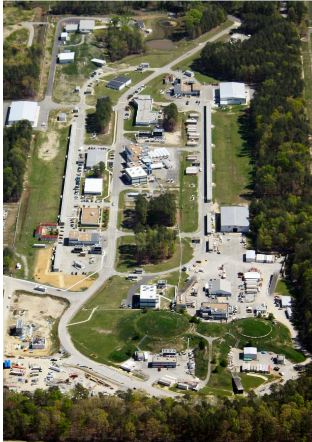
Figure 2.1: An aerial view of CEBAF is shown with the race-track configuration of the accelerator. Hall B is seen at the bottom of the figure, in the middle of the three mounds (circular grass-covered hills), between Halls A and C. Figure taken from [71].
