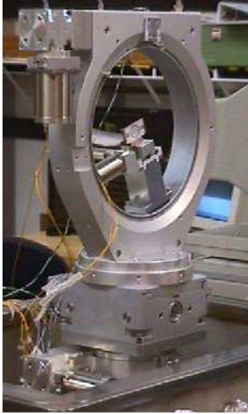
Figure 2.8: The Hall-B goniometer. The target ladder, which holds the various radiators, is in the center of the device. Figure taken from [71].
